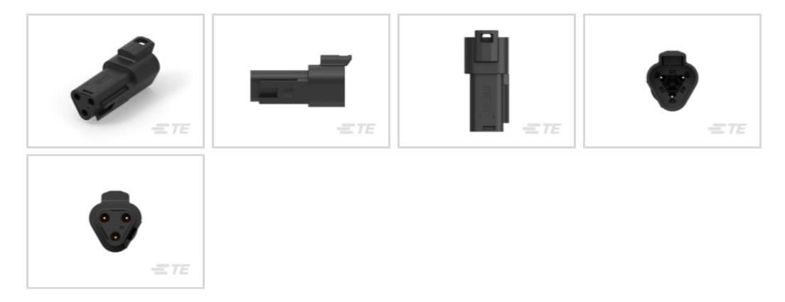
Connector & Housing Type: Receptacle Mating Pin Diameter: 1.56 mm [.061 in] Connector System: Wire-to-Wire Number of Positions: 3 Centerline (Pitch): 8.66 mm [.34 in]
