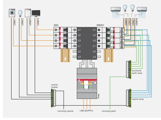
Example of installation of DSE201 in a distribution board (chassis) in conjunction with other ABB protection devices.
