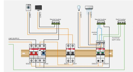
Example of installation of DSE201 in a consumer unit (DIN rail) in conjunction with other ABB protection devices.
