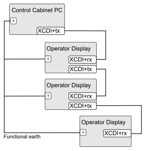
Fig. 10-22: Wiring up to three operating displays using CDI+ at a control cabinet PC
