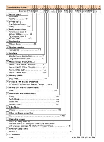
Fig. 15-1: Type code for PR31 devices
