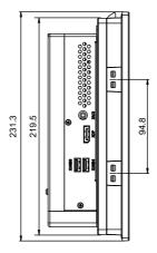
Fig. 10-7: Housing dimensions of the device VR3112, left side view
