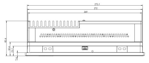
Fig. 10-6: Housing dimensions of the device VR3110, top view
