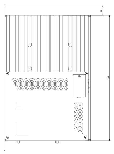
Fig. 10-2: Housing dimensions, left side view
