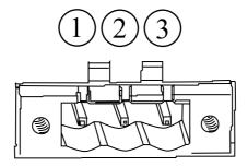
Fig. 9-3: Interface for 24 V voltage supply
