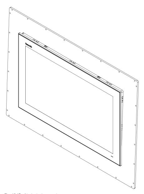
Fig. 10-17: Display in the mounting cut-out
