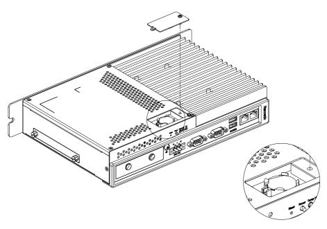
Fig. 10-14: Replacing the CMOS battery
