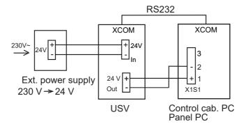
Fig. 10-23: Overall connection diagram - Power supply unit, UPS and control cabinet PC
