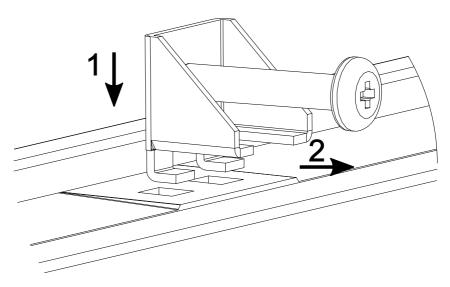
Fig. 10-18: Inserting fastening element into the opening
