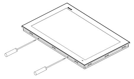
Fig. 10-15: Mounting screws at the bottom of the display
