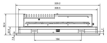
Fig. 10-8: Housing dimensions of the device VR3112, top view
