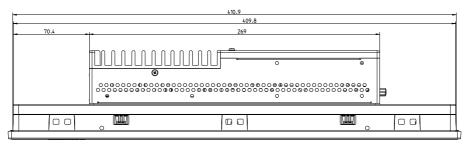
Fig. 10-10: Housing dimensions of the device VR3115, top view
