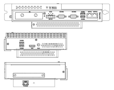
**Fig. 9-2:** Interfaces PR31 with CDI+ interface. At the front side (up), at the upper housing site (middle), the mass memory slot and the CDI+ interface at the bottom of the housing (down).
