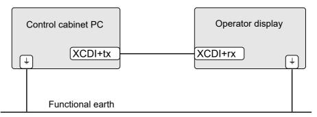
Fig. 10-21: Wiring the control cabinet PC to the operating display
