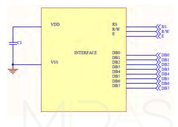
Pin connected to MCU interface: RS, R/W, E, DB0~7
