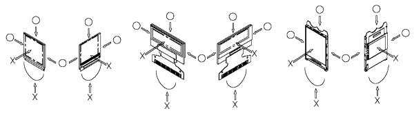
(9) Do not apply stress to the LSI chips and the surrounding molded sections.
