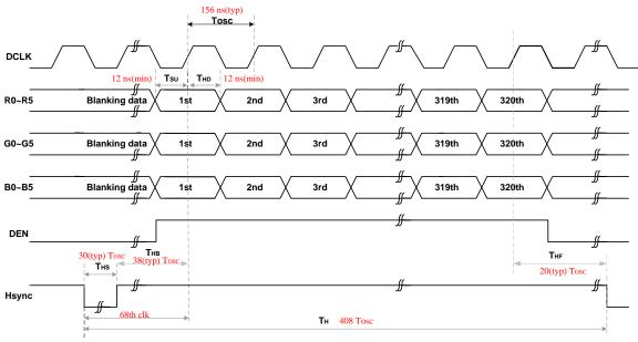
If DEN is fixed to low, the SYNC mode is used. Otherwise DE mode is used. When SYNC mode is used, 1st data start from 68th CLK after Hsync falling
