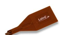
This NFC flex PCB antenna is included with the DVK-BL6xx products. It was tested with the BL65xx series of modules for NFC applications and use.
