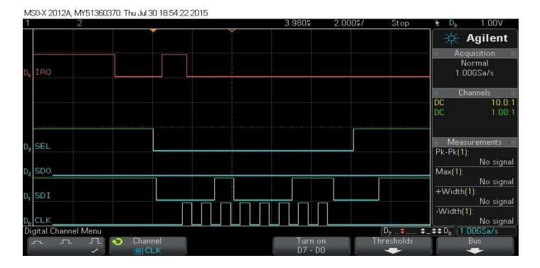
Above is the first byte of SPI data following U IRQ going low after an RF packet has been received.
