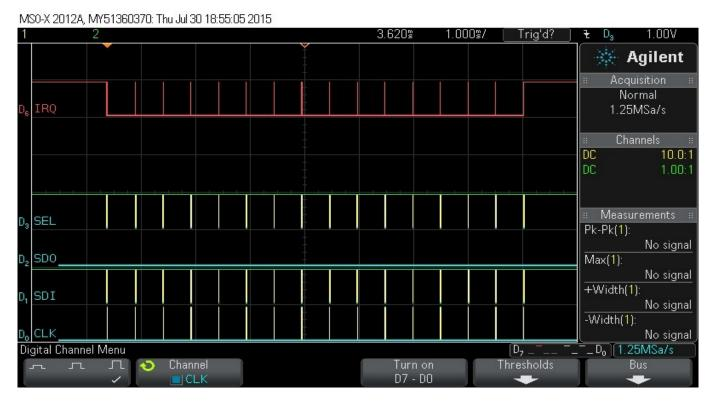
Above is the complete SPI & IRQ Timing diagram for #R<RSSI> <Packet > plus 12 byte data packet
