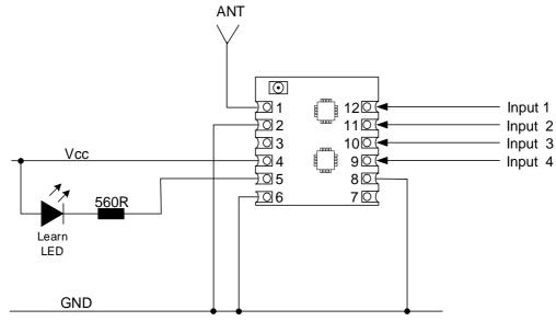
Note: in this example The AUTOMAP and Acknowledge are both activated shown connected.
