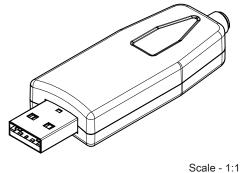
CHECKED REVISION DATE (YYYY-MM-DD) GENERAL TOLERANCE PROJECTION METHOD GE 001.024 2019-07-18 DIN ISO 2768-1m WIRL-PR09 Radio module 915MHz Würth Elektronik eiSos GmbH & Co. KG low power 2607056291011 Tel. +49 (0) 79 42 945 - 0 www.we-online.com BUSINESS UNIT STATUS PAGE 1/4 eiSmart Valid
