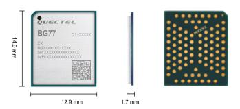
BG77 is an ultra-compact LPWA module supporting LTE Cat M1, LTE Cat NB2 and integrated GNSS. It is fully compliant with 3GPP Rel-14 specification and provides maximum data rates of 588 kbps downlink and 1119 kbps uplink. It features ultra-low power consumption by leveraging the integrated RAM/flash as well as the ARM Cortex A7 processor supporting ThreadX, achieving up to 70% reduction in PSM leakage and 85% reduction in eDRX current consumption compared to its predecessor.
