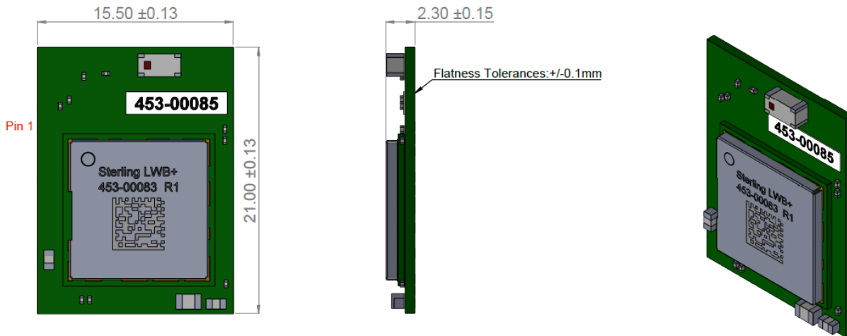
Figure 18: Sterling LWB+ MHF® 4 and chip antenna module dimension
