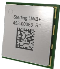
Figure 1: Sterling LWB+ base SiP module (453-00083)
