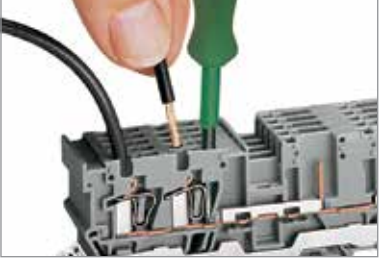
Carrier terminal block: Terminating/removing conductor via operating tool (3.5 x 0.5 mm blade).
