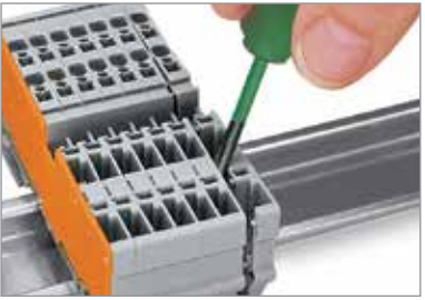
Open assembly by laterally sliding terminal block via operating tool, then snap off terminal block from the rail.
