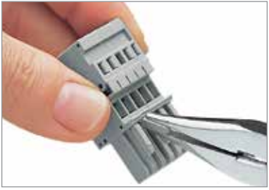
Coding a female plug by removing coding finger(s). Do not remove the first and last coding fingers or use additional locking lever.
