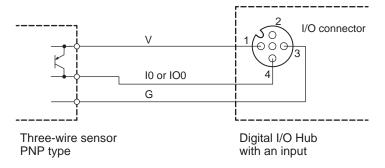
The power to pin 1, or +(V), is supplied from the IO-Link Master Unit through the IO-Link cable to the Digital I/O Hub.
