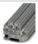
Double-level spring-cage terminal block, connection method: Spring-cage connection, cross section:  $0.08 \text{ mm}^2$  -  $4 \text{ mm}^2$ , AWG: 28 - 12, width: 5.2 mm, color: gray, mounting type: NS 35/7,5, NS 35/15
