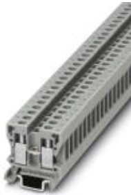
Mini feed-through terminal block, Connection method: Screw connection, Cross section: 0.2 mm 2 - 2.5 mm 2 , AWG: 24 - 14, Width: 5.2 mm, Color: gray, Mounting type: NS 15
