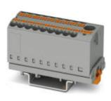
Distribution block, Block with vertical alignment and integrated supply, Connection method: Push-in connection, Push-in connection, Number of connections: 19, Cross section: 0.14 mm<sup>2</sup> - 4 mm<sup>2</sup>, AWG: 26 - 12, Width: 28.6 mm, Height: 28.7 mm, Color: gray, Mounting type: NS 35/7,5, NS 35/15
