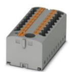
Distribution block, Basic terminal block with supply, Connection method: Push-in connection, Push-in connection, Number of connections: 19, Cross section: 0.14 mm² - 4 mm², AWG: 26 - 12, Width: 56 mm, Height: 21.2 mm, Color: gray, Mounting type: Adhesive
