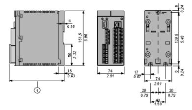
When using XPSMCTS• connectors this dimension is 153 mm (6.02 in) When using XPSMCTC• connectors this dimension is 151,5 mm (5.96 in)
