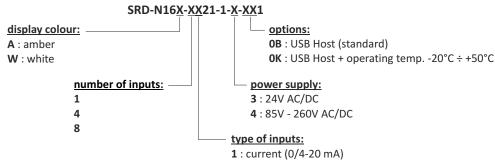
2: voltage (0/1-5 V, 0/2-10V) 3: RTD (Pt100, Pt500, Pt1000) A: thermocouple (K, S, J, T, N, R, B, E)
