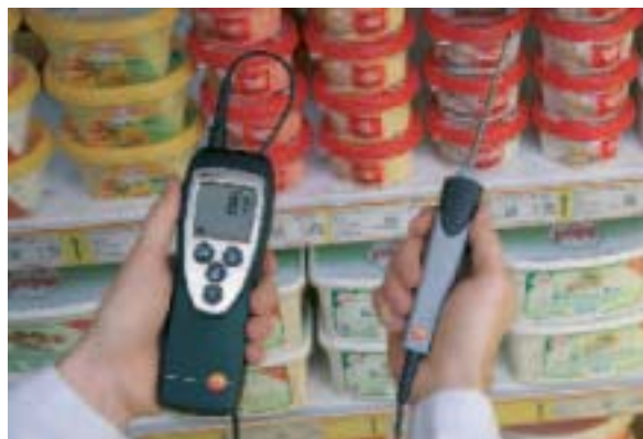
Inspects a refrigerated counter for sufficient refrigeration power
