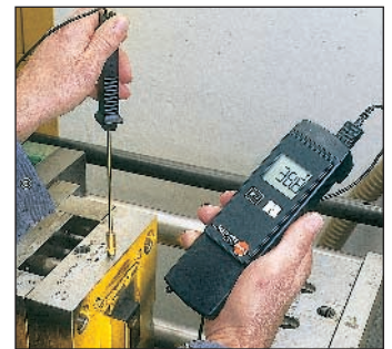
Surface temperature in moulding tools
