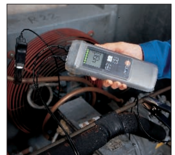
Measures superheating or sub cooling in refrigeration systems
