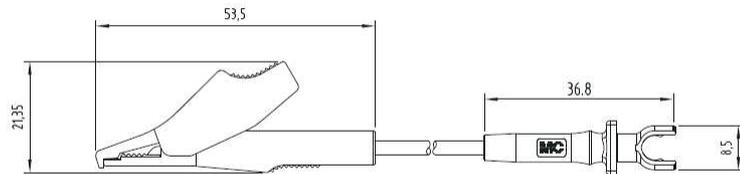
Highly flexible reference lead with insulation in Silicone. One end with fork-type plug for connecting to the shielded contact on the side of the probe, other end with crocodile clip with all-round insulation and toothed gripping jaws with fine-wire clamping surface.
