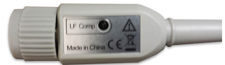
Figure 2. Low-frequency compensation adjustment (for N2840A/41A/42A/43A/53A)
