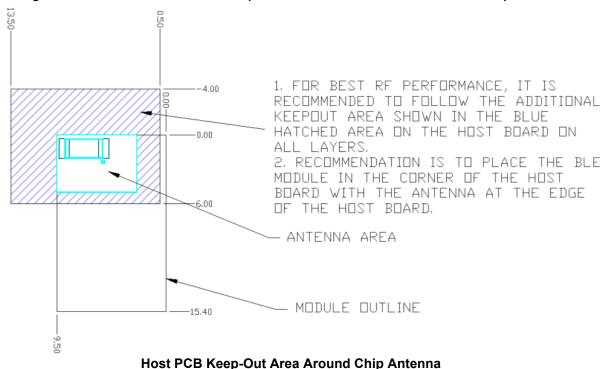
Figure 3. Recommended Host PCB Keep-Out Area Around the CYBLE-224110-00 Chip Antenna
