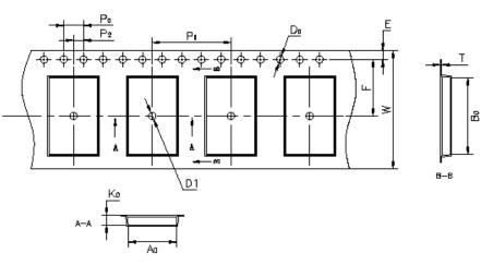
Figure 11 details the orientation of the CYBLE-224110-00 in the tape as well as the direction for unreeling.
