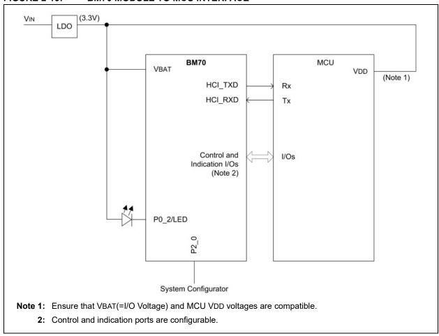
FIGURE 2-11: BM71 MODULE TO MCU INTERFACE
