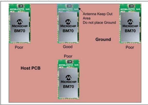
Figure 4-4 illustrates a typical example of the good and poor antenna placement of the BM71BLES1FC2 module on the main application board with the ground plane.
