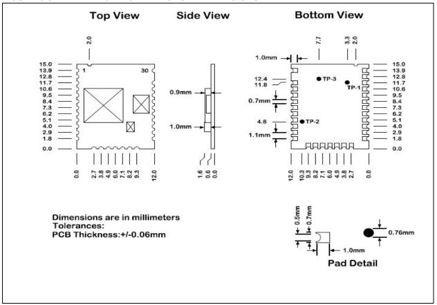
Figure 6-4 illustrates the recommended PCB footprint.
