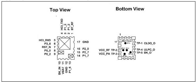
FIGURE 1-6: BM71BLES1FC2 PIN DIAGRAM
