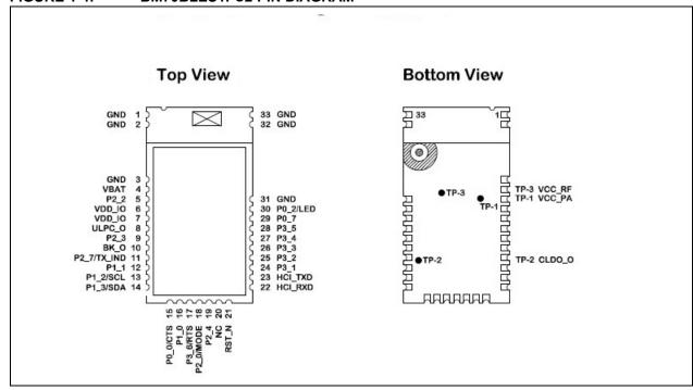
FIGURE 1-5: BM71BLE01FC2 PIN DIAGRAM
