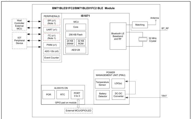
**Note 1:** SPI and I<sup>2</sup>C peripherals of the IS1870/71 IC can be enabled on the BM70/71 module by changing the default firmware. For more details, contact a local Microchip representative.
