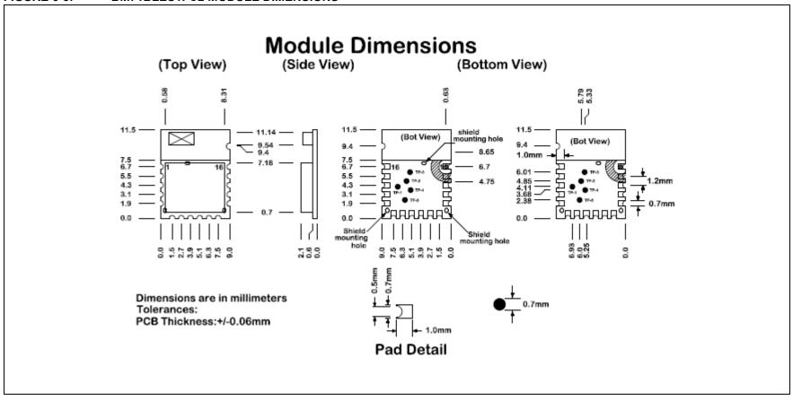
Figure 6-6 illustrates the recommended PCB footprint. Ensure that no top copper layer is near the test pin area.
