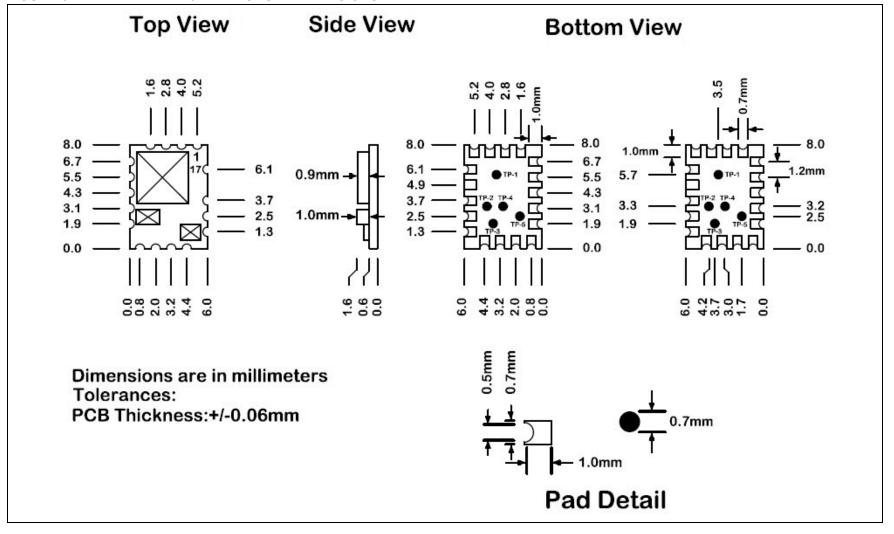
Figure 6-8 illustrates the recommended PCB footprint.
