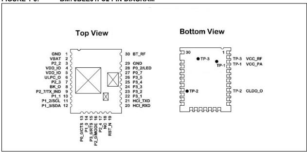
FIGURE 1-4: BM70BLES1FC2 PIN DIAGRAM
