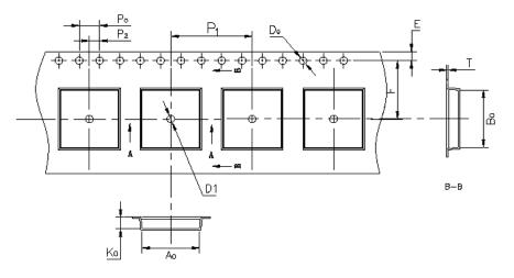
Figure 11 details the orientation of the CYBLE-014008-00 in the tape as well as the direction for unreeling.
