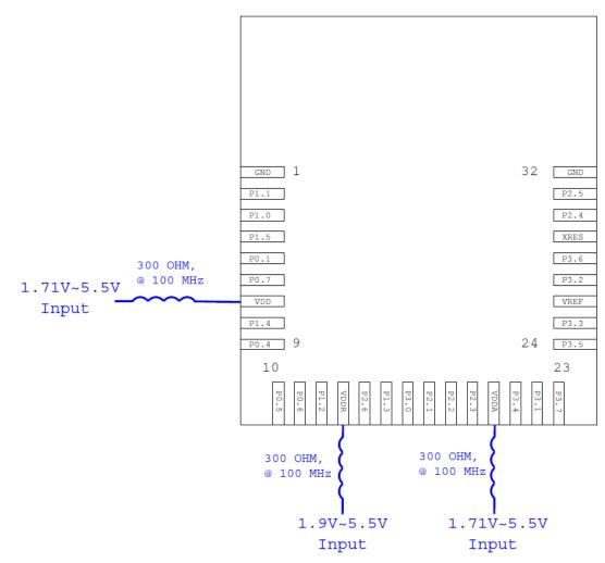
Figure 8. Recommended Host Schematic for Independent Supply Option
