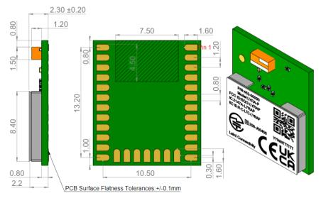
Figure 11: Module dimensions (mm)
