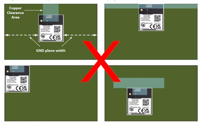
Figure 10: Non-optimal layout examples
