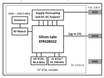
Figure 1: Lyra P Block Diagram
