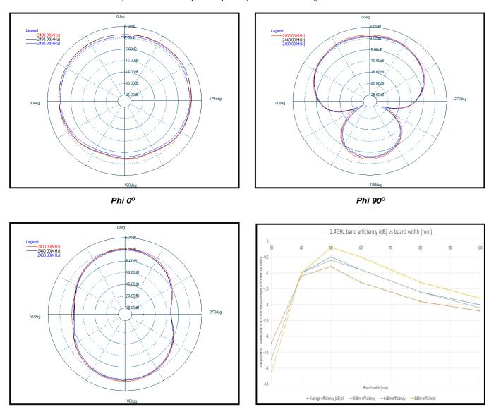
Figure 5: Typical 2D Antenna Radiation Patterns and Efficiency
