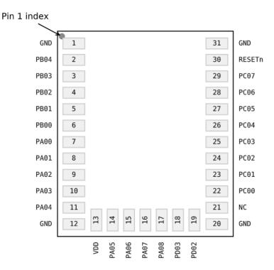
Figure 8: Lyra P 31-Pin PCB Module With LF Crystal Device Pinout
