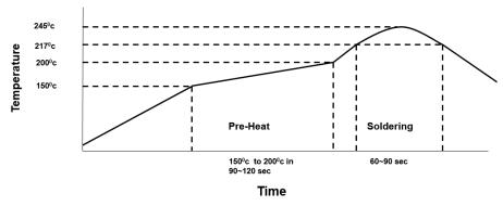
Figure 14: Recommended Reflow Profile
