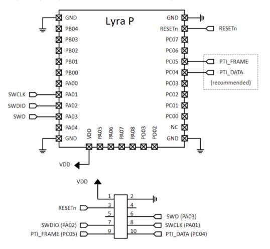
Figure 7: Stand-Alone SoC Configuration
