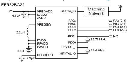
Figure 2: Lyra P Module Schematic
