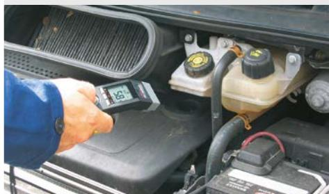
Check temperatures of engines and catalytic converters, scan ignition system problems, analyse cooling system restrictions, diagnose air conditioning systems, check tyres and brakes with uneven braking.
