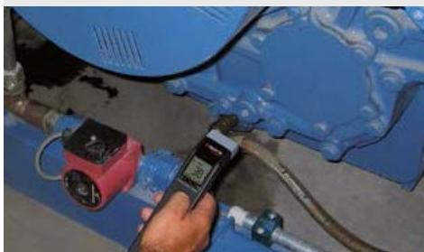
Observe temperatures of motors and drives, bearings and valves. Gather temperature data of heating and ventilation components. Check furnace performance and steam distribution systems.
