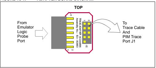
FIGURE 16-2: ADAPTER BOARD PIN CONNECTION DIAGRAM
