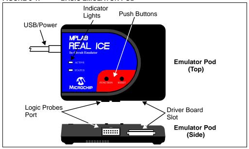
The emulator communicates with the PC and is powered through the USB cable.
