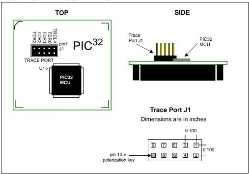
FIGURE 15-2: PIC32 PIM PIN CONNECTION DIAGRAM
