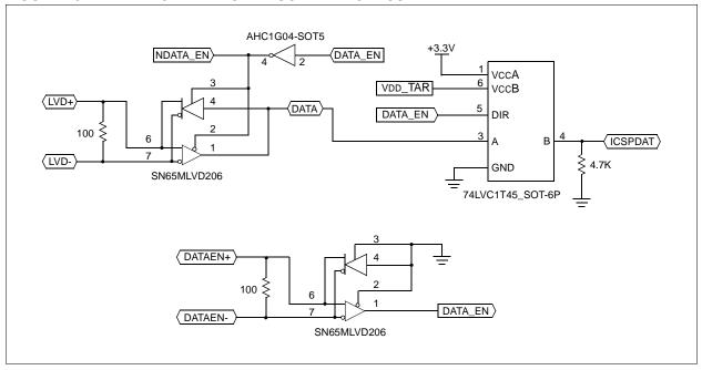
FIGURE 13-5: RECEIVER BOARD SCHEMATIC – ICSPCLK
