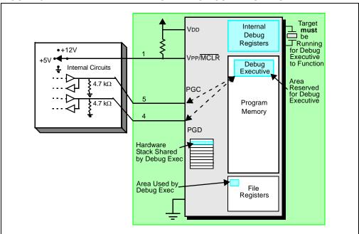
Typically, in order to find out if an application program will run correctly, a breakpoint is set early in the program code. When a breakpoint is set from the user interface of MPLAB IDE, the address of the breakpoint is stored in the special internal debug registers of the target device. Commands on PGC and PGD communicate directly to these registers to set the breakpoint address.
