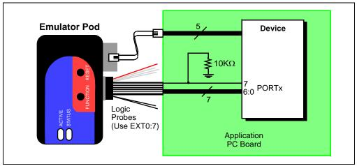
For this trace configuration, seven (7) lines of data and one (1) line for clock are transmitted. PORTx must be a port with eight pins that has all eight pins available for trace. The port does not have to be one physical port but can be made up of pins from more than one port. The port pins must not be multiplexed with the currently-used PGC and PGD pins.
