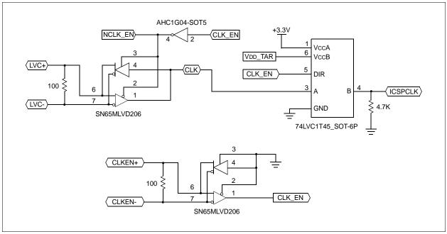
FIGURE 13-6: RECEIVER BOARD SCHEMATIC – DAT & CLK
