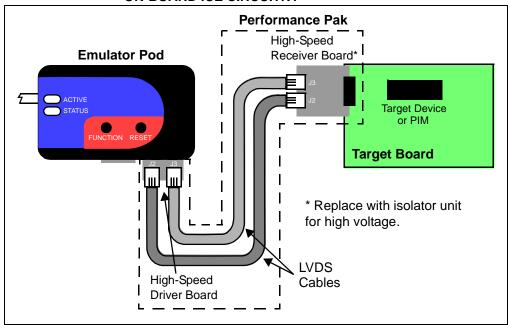
FIGURE 3-5: HIGH-SPEED/LVDS CONNECTION – ICE DEVICE
