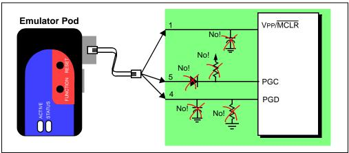
**VPP/MCLR pin:** do not use capacitors on  $\overline{MCLR}$  – they will prevent fast transitions of VPP. A simple pull-up resistor is generally sufficient.
