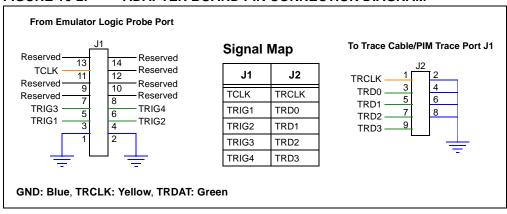
**FIGURE 16-3:** TRACE CABLE DIAGRAM From To Adapter PIM Trace Board **BOTTOM** Port J1 Port J2 Pin 1 Pin 1 SIDE
