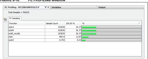
FIGURE 6-10: PC PROFILING WINDOW
