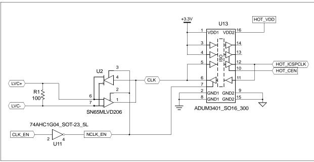
FIGURE 17-4: ISOLATOR UNIT SCHEMATIC – DAT & CLK
