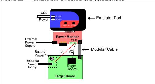
FIGURE 23: POWER MONITOR BOARD CHB CONNECTIONS
