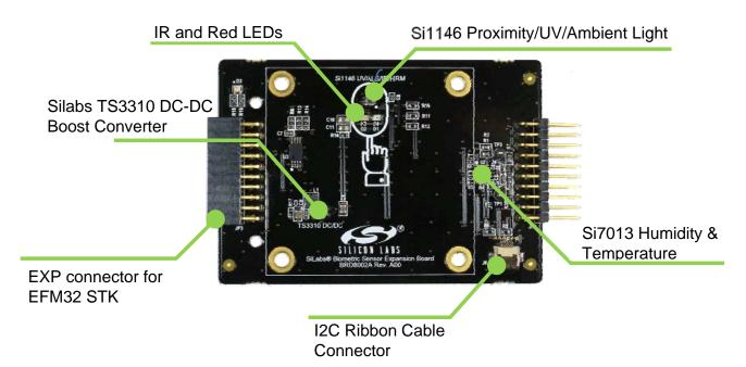
Figure 13. Biometric-EXP Hardware Component Layout
