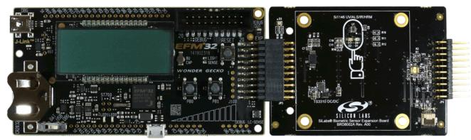
Figure 1. EFM32 Wonder Gecko STK (Left) Connected to a Biometric-EXP (Right)
