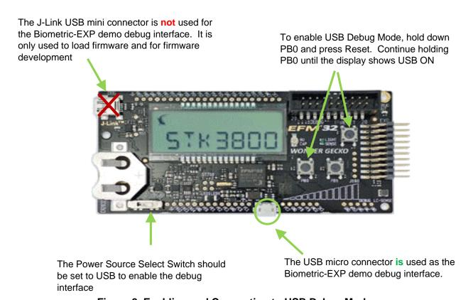
Figure 8. Enabling and Connecting to USB Debug Mode
