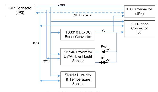
Figure 12. Biometric-EXP Block Diagram
