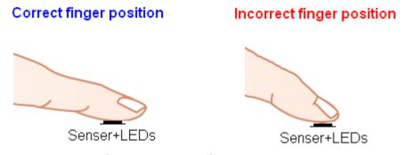
Figure 7. Proper Finger Placement
