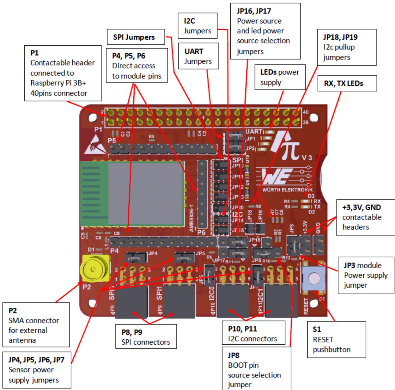
Figure 20: Top view (mounted on Raspberry Pi 3B)
