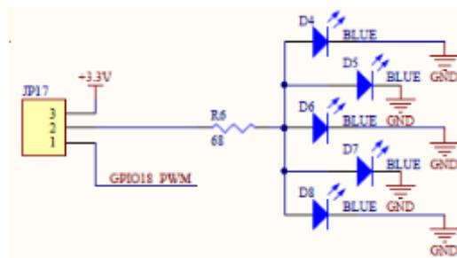
Figure 32: POWER SUPPLY leds
