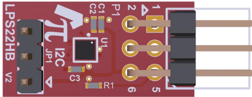
Figure 17: LPS22HB sensor board
