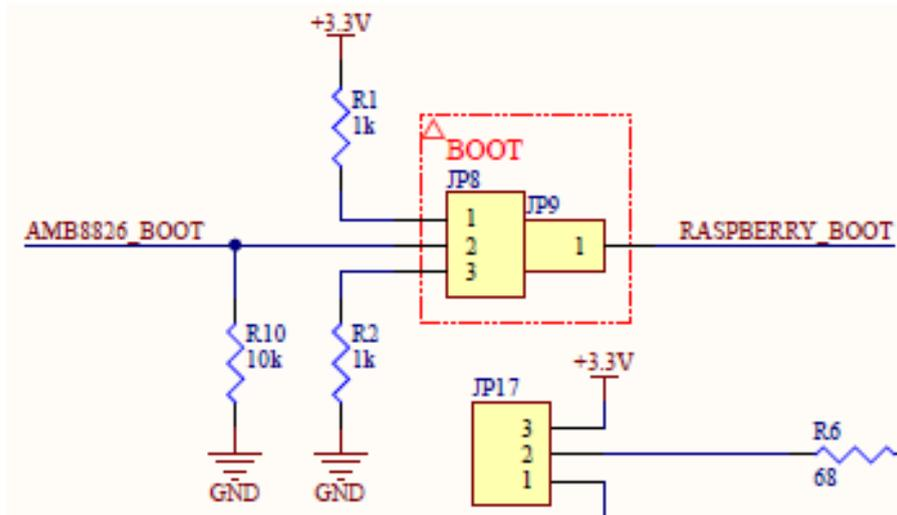
Figure 29: BOOT pin connections
