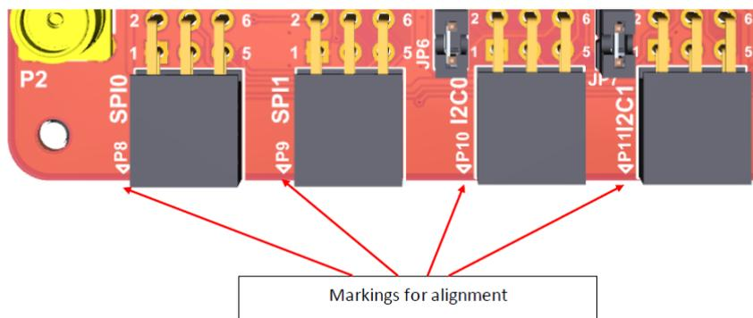
Figure 22: Sensor boards alignment
