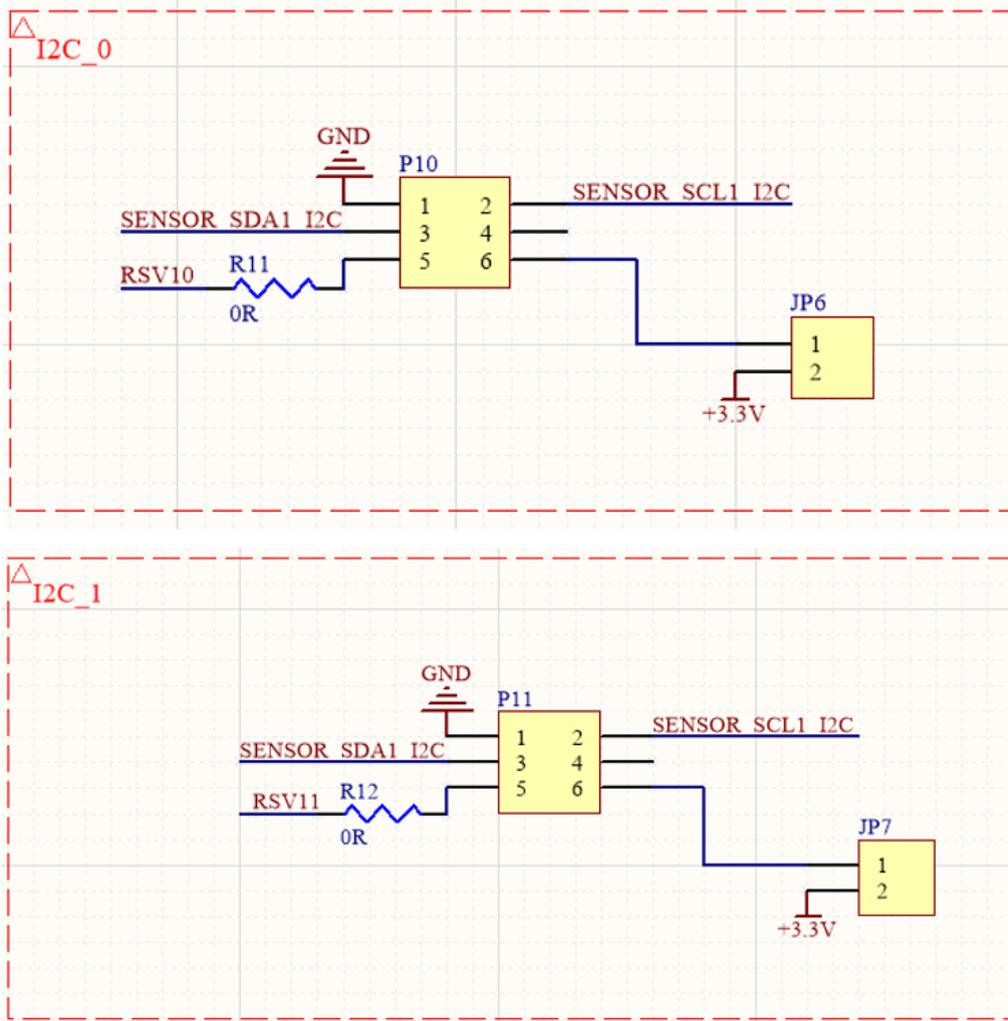
Figure 28: I2C connectors P10 and P11
