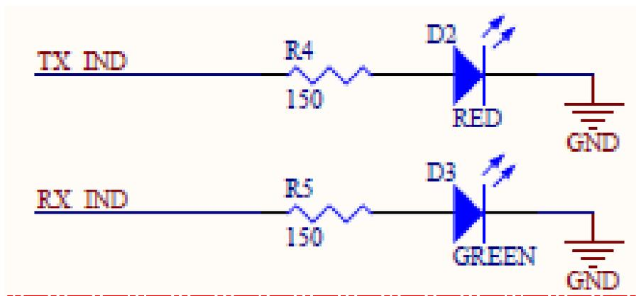
Figure 31: TX and RX leds
