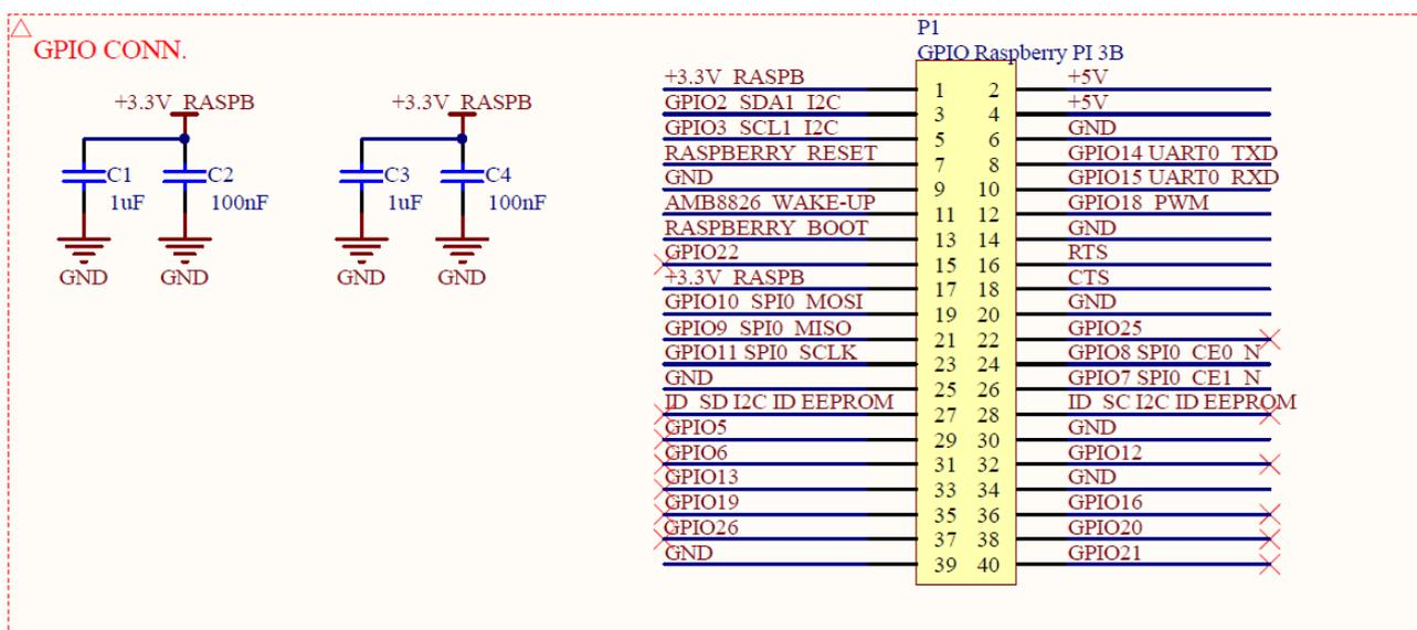
Figure 25: Extended connector P1 from Raspberry Pi board
