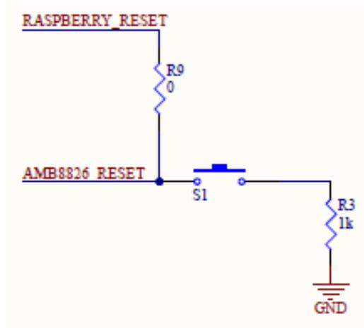
Figure 30: RESET pin connections
