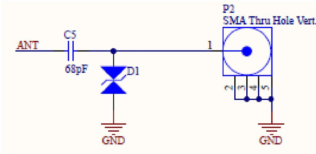
Figure 26: SMA connector P2 for external antenna connection
