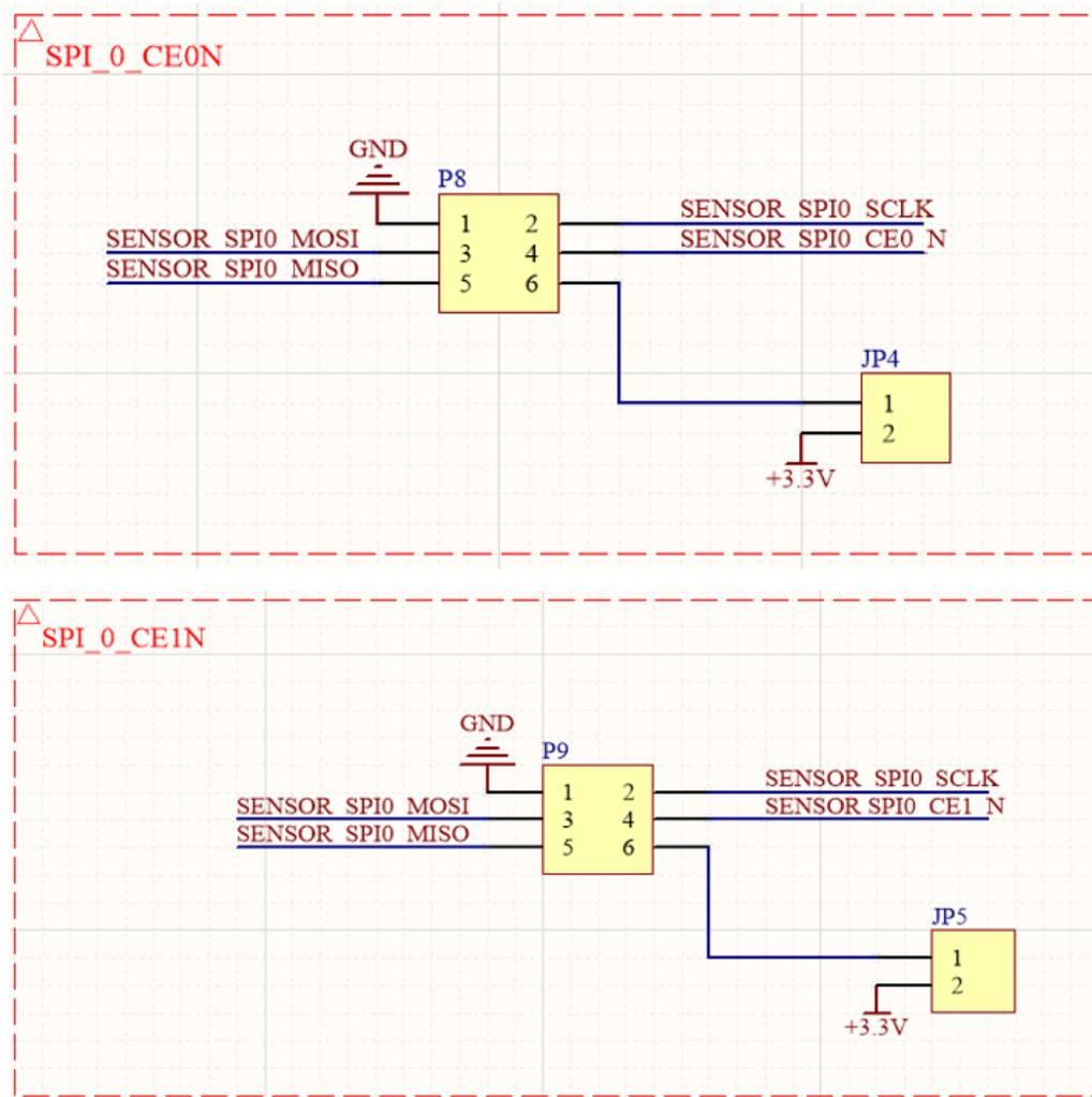
Figure 27: SPI connectors P8 and P9
