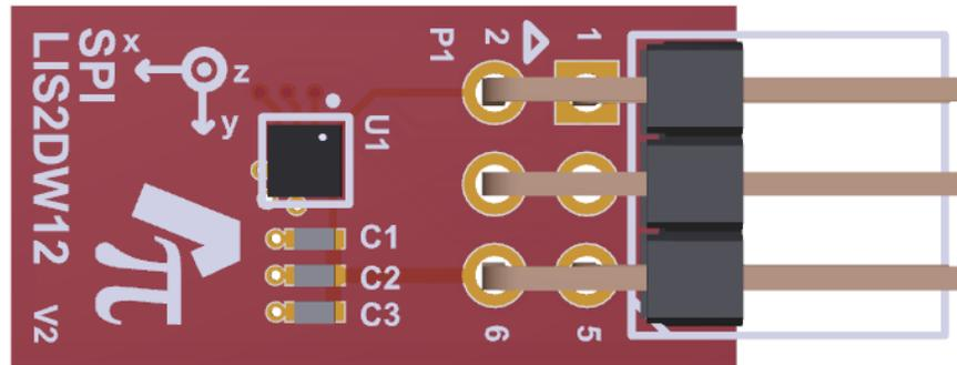
Figure 18: LIS2DW12 sensor board
