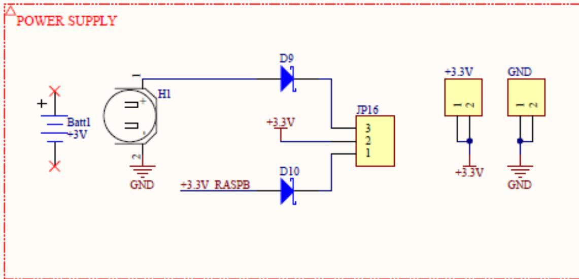
Figure 24: Power supply schematic
