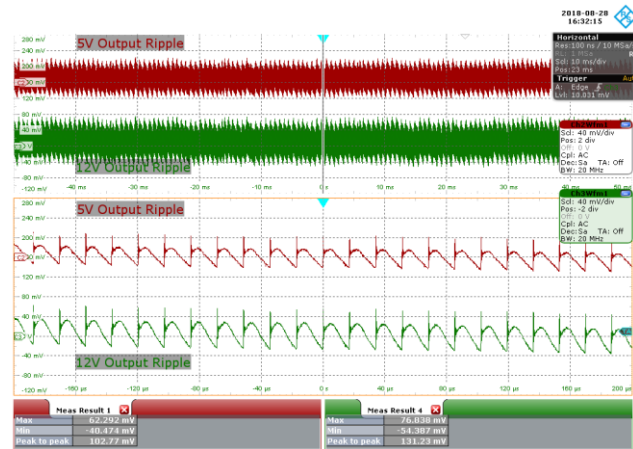
Figure 111 – 115 VAC 60 Hz, 100% Load. CH2: 5 V OUT , 40 mV / div., 10 ms / div. CH3: 12 V OUT , 40 mV / div., 10 ms / div. Zoom: 40 μs / div. 5 V Output Ripple = 134.39 mV. 12 V Output Ripple = 156.62 mV.
