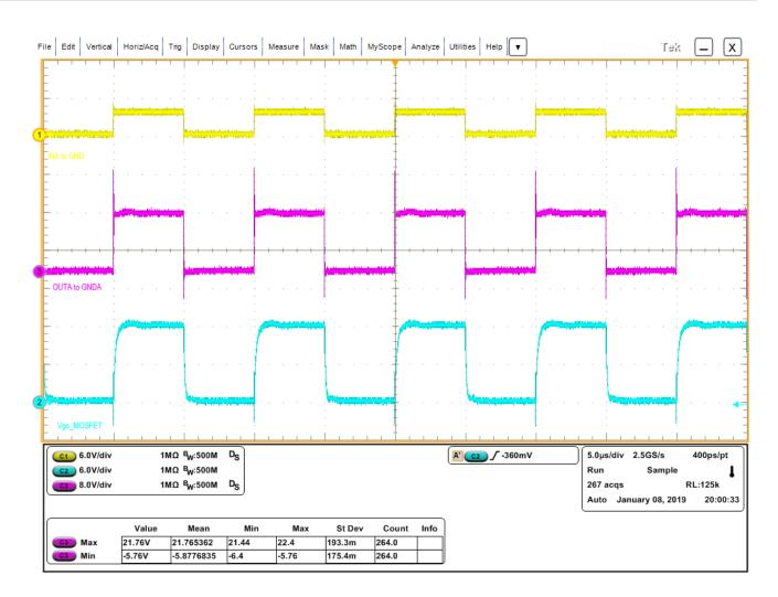
Measurements done on a single MOSFET with  $V_{DS} = 0 V$  (drain and source shorted)
