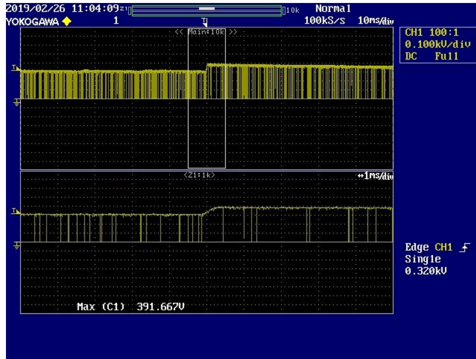
Figure 40 – Drain Voltage, 230 VAC, Full Load.
