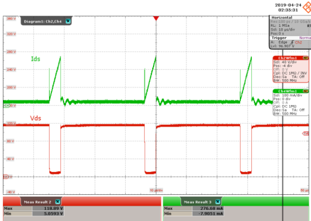
Figure 14 – Drain Voltage and Current Waveforms. 85 VAC, 120 mA Output. Upper: I_{DRAIN} , 100 mA / div. Lower: V_{DRAIN} , 40 V, 10 \mu s / div. I_{MAX} = 276.7 mA, V_{MAX} = 118.9 V.
