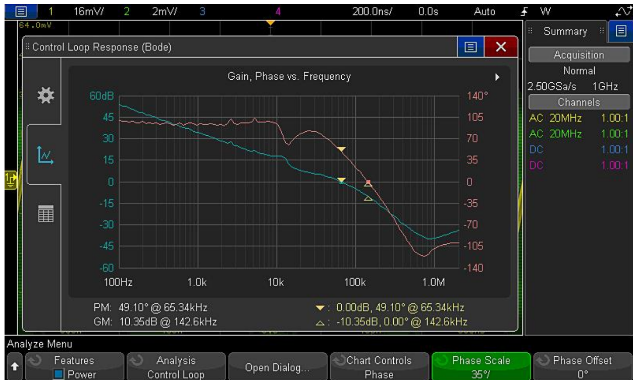
Figure 34. Control loop response analysis (bode plot) shows the gain/phase plot over frequency sweep range up to 20 MHz with automatic determination of phase margin (PM) and gain margin (GM).
