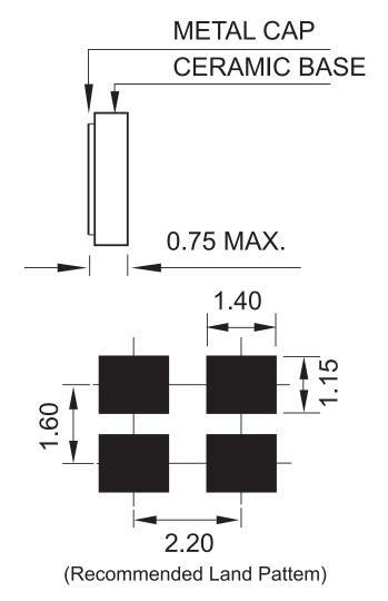
Package is Seam Sealed Ceramic-Metal. Dimensions are millimeters.
