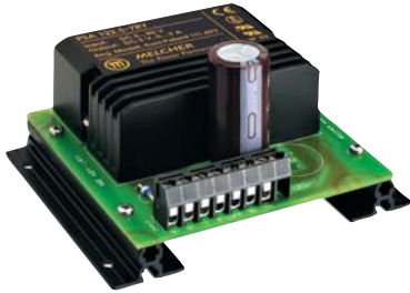
Fig. 16 Adapter for chassis mounting
