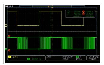
CH1: PWM Pin Voltage CH4:OUT1/2 Current Figure 4: Internal PWM Dimming
