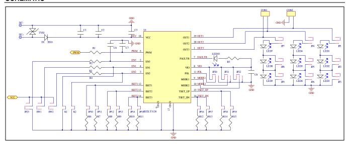
Figure 5: IS32LT3128/3128A DEMO Board Schematic
