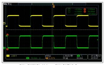
CH1: PWM Pin Voltage CH4:OUT1/2 Current Figure 3: External PWM Dimming (Negative Polarity)
