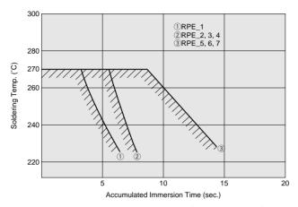
Perform soldering within tolerance range (shaded portion).
