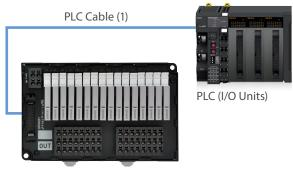
G70V I/O Relay Terminal (One Block, 16 points)
