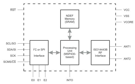
Figure 5-1. Functional Block Diagram
