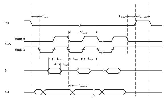
Figure 4-2. SPI Mode Timing
