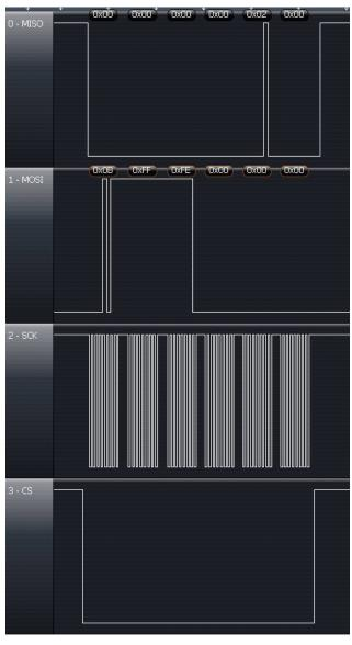
Figure 5-9. SPI Access Example: Read of the Control Register at Address 0xFFFE, Responds With 0x00, 0x02 (RF Enable = 1)
