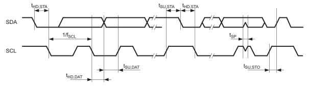
Figure 4-1. I<sup>2</sup>C Mode Timing
