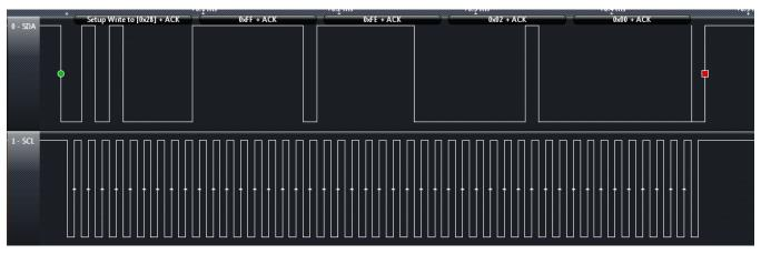
Figure 5-4. I<sup>2</sup>C Access Example: Write of the Control Register at Address 0xFFFE With 0x00, 0x02 (RF Enable = 1)
