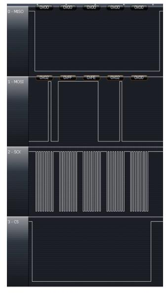
Figure 5-8. SPI Access Example: Write of the Control Register at Address 0xFFFE With 0x00, 0x02 (RF Enable = 1)
