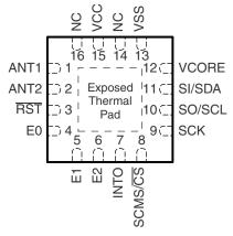
Figure 3-2. 16-Pin RGT Package (Top View)
