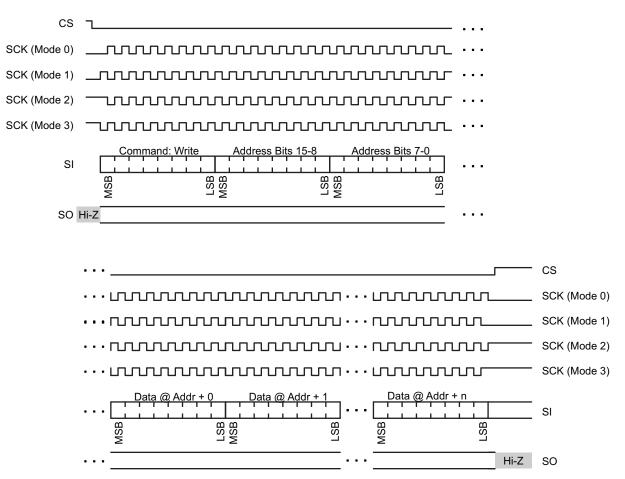
Figure 5-6. SPI Write Access
