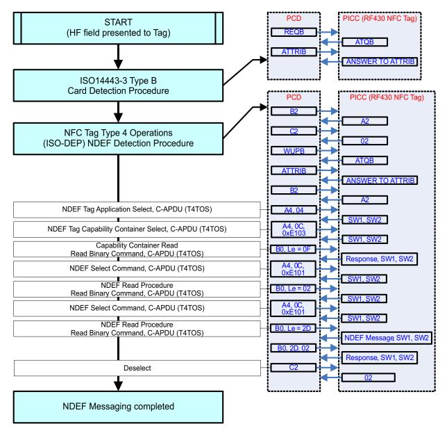
Figure 5-10. Command and Response Exchange Flow
