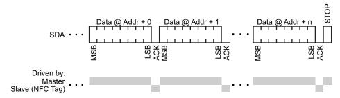
Figure 5-2. I<sup>2</sup>C Write Access
