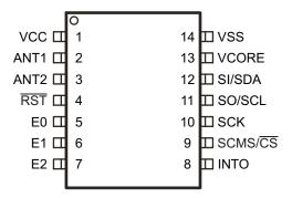
Figure 3-1. 14-Pin PW Package (Top View)
