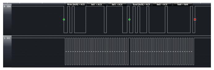
Figure 5-5. I<sup>2</sup>C Access Example: Read of the Control Register at Address 0xFFFE, Responds With 0x00, 0x02 (RF Enable = 1)
