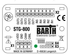
If you choose the Open Source Programming Option, use the X3 connector for programming and debugging via the Connection Cable VK-35 (BARTH® Art. No. 0091-0035). In this case the X4 connector can be used as TTL232 UART interface within your application.
