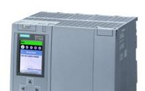
SIMATIC S7-1500T, CPU 1518T-4 PN/DP, central processing unit with 9 MB work memory for program and 60 MB for data, 1st interface: PROFINET IRT with 2-port switch, 2nd interface: PROFINET RT, 3rd interface: PROFINET basic services, 4th interface: PROFIBUS, 1 ns bit performance, SIMATIC memory card required
