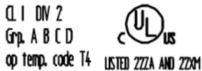
Figure 81: Printing on text detail in accordance with NEC
