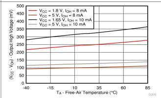
Figure 6-6. Output High Voltage (V<sub>CC</sub> – V<sub>OH</sub>) vs Temperature (T<sub>A</sub>) for P-Ports
