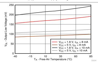
Figure 6-4. Output Low Voltage (V<sub>OL</sub>) vs Temperature (T<sub>A</sub>) for P-Port I/Os
