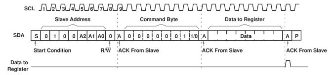
Figure 8-9. Write To Configuration Or Polarity Inversion Registers
