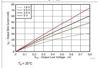
Figure 6-5. Sink Current (I<sub>OL</sub>) vs Output Low Voltage (V<sub>OL</sub>) for P-Ports at Four Supply Voltages
