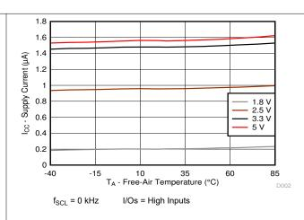
Figure 6-2. Supply Current (ICC, Standby Mode) vs Temperature (T<sub>A</sub>) at Four Supply Voltages
