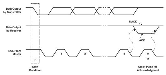
Figure 8-5. Acknowledgment On The I<sup>2</sup>C Bus
