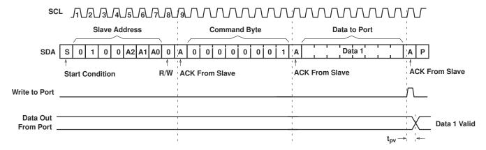
Figure 8-8. Write To Output Port Register
