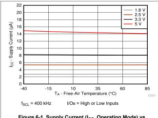
Figure 6-1. Supply Current (I<sub>CC</sub>, Operating Mode) vs Temperature (T<sub>A</sub>) at Four Supply Voltages
