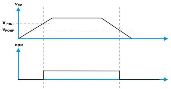
Figure 33. Waveform Describing V<sub>CC</sub> Voltage Level at Which Power-On-Reset (POR) Occurs
