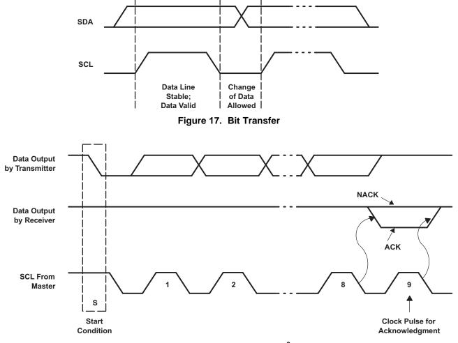
Figure 18. Acknowledgment on I<sup>2</sup>C Bus
