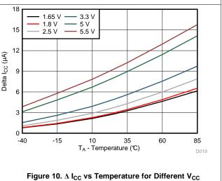
$(V_{I} = V_{CC} - 0.6 V)$
