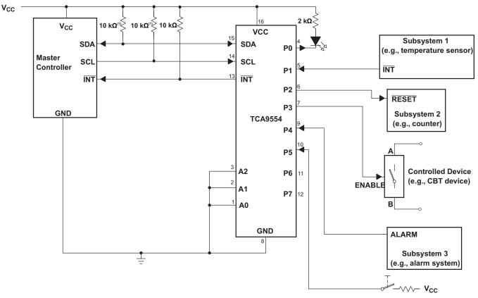
(1) The SCL and SDA pins must be tied directly to VCC because if SCL and SDA are tied to an auxiliary power supply that can be powered on while VCC is powered off, then the supply current, ICC, will increase as a result.
