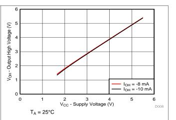
Figure 7. Source Current (I<sub>OH</sub>) vs Output High Voltage (V<sub>OH</sub>)
