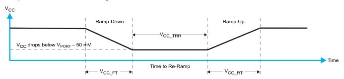
Figure 31. V<sub>CC</sub> is Lowered Below the POR Threshold, Then Ramped Back Up to V<sub>CC</sub>
