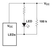
Figure 27. High-Value Resistor in Parallel With LED
