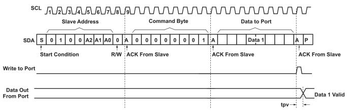
Figure 23. Write to Output Port Register
