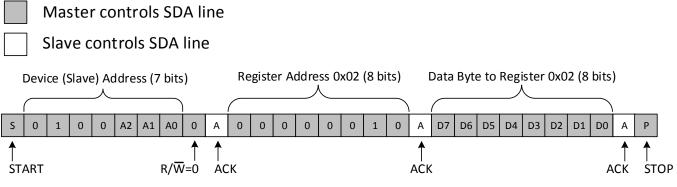
Figure 22. Write to the Polarity Inversion Register
