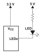
Figure 28. Device Supplied by a Lower Voltage
