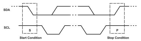
Figure 16. Definition of Start and Stop Conditions
