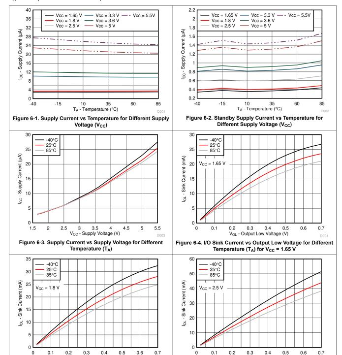
$V_{OL} \mbox{-} \mbox{Output Low Voltage (V)}$  Figure 6-5. I/O Sink Current vs Output Low Voltage for Different
