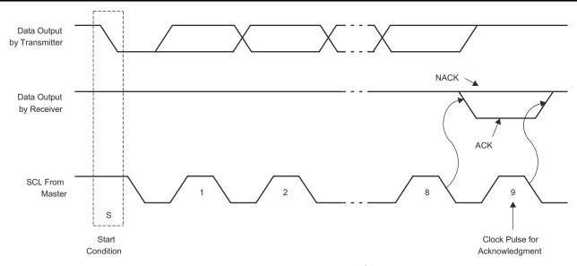
Figure 8-5. Acknowledgment On I<sup>2</sup>C Bus
