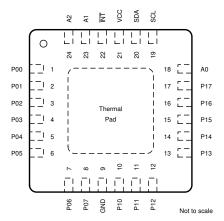
Figure 5-2. RGE Package, 24 Pin (QFN), (Top View)
