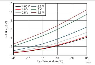
Figure 6-18.  $\Delta$  I<sub>CC</sub> vs Temperature for Different V<sub>CC</sub> (V<sub>I</sub> = V<sub>CC</sub> - 0.6 V)
