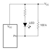
Figure 9-2. High-Value Resistor In Parallel With Led
