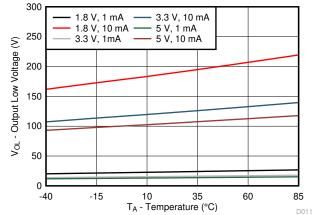
Figure 6-9. I/O Sink Current vs Output Low Voltage for Different Temperature  $(T_A)$  for  $V_{CC}$  = 5.5 V
