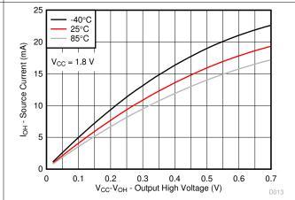
Figure 6-11. I/O Source Current vs Output High Voltage for Different Temperature ( $T_A$ ) for  $V_{CC}$  = 1.65 V
