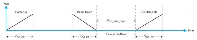
Figure 10-1. V<sub>CC</sub> Is Lowered Below 0.2 V Or 0 V And Then Ramped Up To V<sub>CC</sub>
