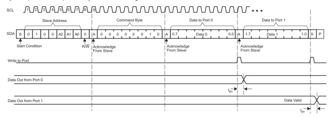
Figure 8-8. Write To Output Port Registers
