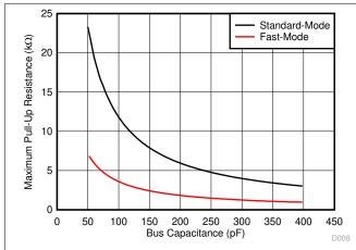
Standard-mode:  $f_{SCL}$  = 100 kHz,  $t_r$  = 1  $\mu s$  Fast-mode:  $f_{SCL}$  = 400 kHz,  $t_r$  = 300 ns
