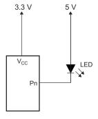
Figure 9-3. Device Supplied By Lower Voltage
