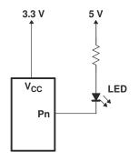
Figure 9-3. Device Supplied By Lower Voltage
