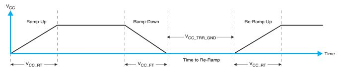
Figure 10-1. V<sub>CC</sub> Is Lowered Below 0.2 V Or 0 V And Then Ramped Up To V<sub>CC</sub>
