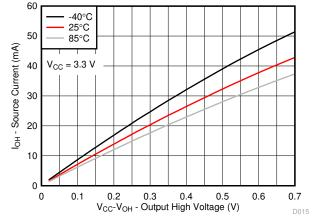
Figure 6-14. I/O Source Current vs Output High Voltage for Different Temperature (T<sub>A</sub>) for V<sub>CC</sub> = 3.3
