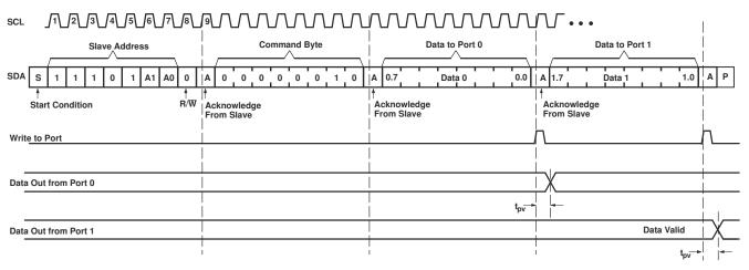
Figure 8-8. Write To Output Port Registers
