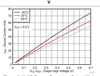
Figure 6-15. I/O Source Current vs Output High Voltage for Different Temperature (T<sub>A</sub>) for V<sub>CC</sub> = 5 V
