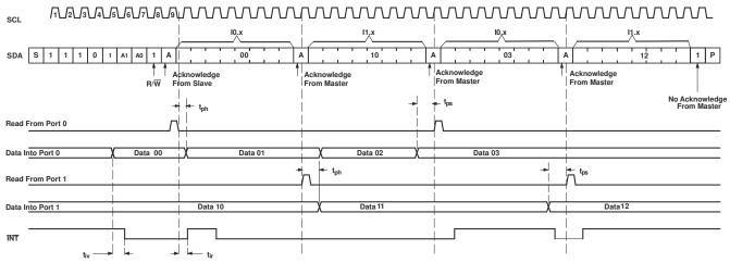
A. Transfer of data can be stopped at any time by a Stop condition. When this occurs, data present at the latest acknowledge phase is valid (output mode). It is assumed that the command byte previously has been set to 00 (Read Input Port register).
