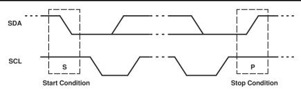
Figure 8-3. Definition Of Start And Stop Conditions
