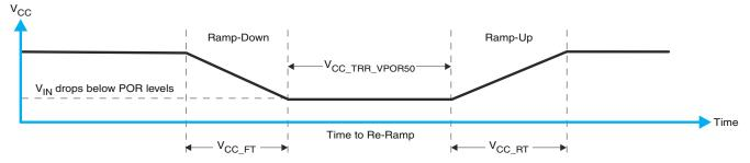
Figure 10-2. V<sub>CC</sub> Is Lowered Below The Por Threshold, Then Ramped Back Up To V<sub>CC</sub>
