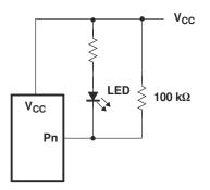
Figure 9-2. High-Value Resistor In Parallel With Led
