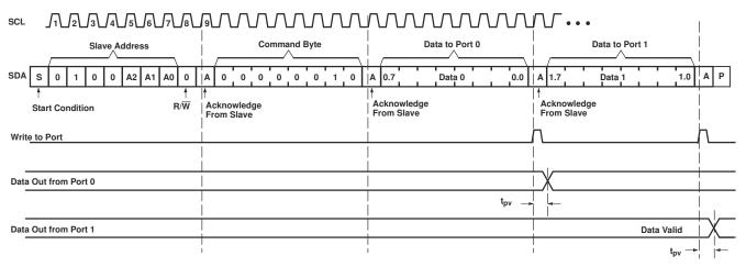
Figure 8-8. Write To Output Port Registers
