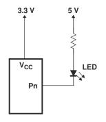
Figure 9-3. Device Supplied By Lower Voltage
